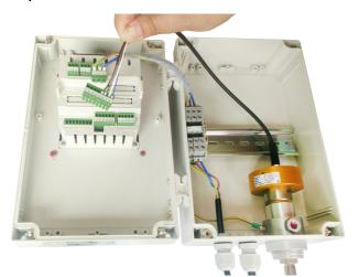
Open the S305 case and remove the sensor cable connected at the display terminal first. See the left picture. To do this, disconnect the entire plug.
