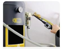
Scan with the focus tube and focus tip the roughly location till the exact location is found.
