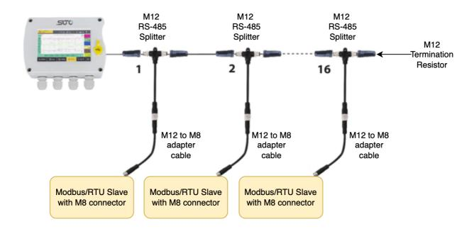
**Remark**: The S331 can maximum provide 10 W power to the connected devices. If more power is required a separate power supply is needed.
