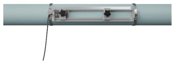
6. Put the other flow transducer from top of the fixture. Make sure that the distance between the two transducers is the "Transducer spacing" value shown on the mobile phone App. Rotate the knob to fix.
