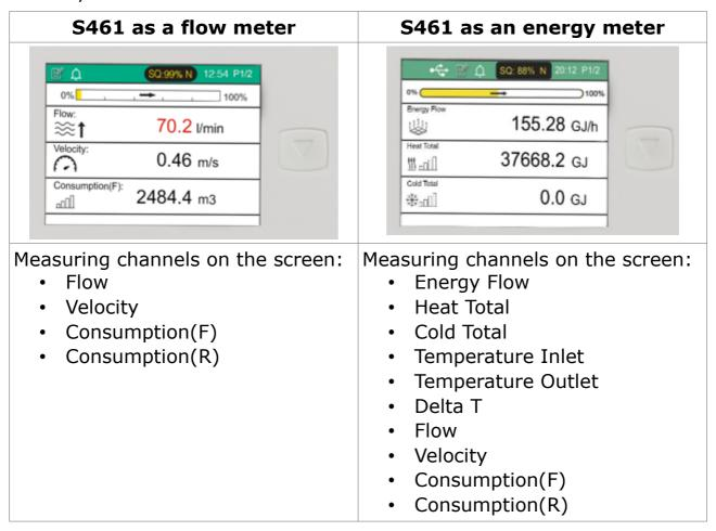
Some measurements have upper limits; for details, see the range column of the **Resolution and units** table in the *S461 Modbus Register Table* IM.
