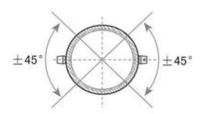
If the Z-Method is used, make sure that the transducers are mounted on a pipe within a valid angle range, as shown in the left picture.
