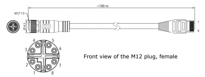
The 8-position pin/pair assignment on the RJ-45 side must comply with the T568B wiring method. The S461 does not support the T568A wiring method.
