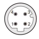
4-pole connector, male (View onto the connector)
