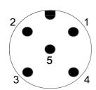
5-pole connector, male (View onto the connector)
