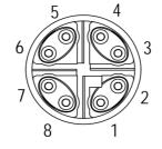
8-pole connector for Ethernet connection, male (View onto the connector)
