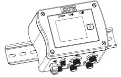
2. Connect the transducers, the power supply and temperature sensors to the designated connectors, as described in the table below.
