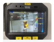
Simply hold the trigger button to capture images. Add voice memos and message notes for each leak.
